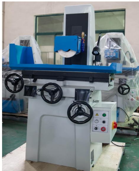
Figure 4: Hydraulic sliding X-axis, automatically driven Y-axis and Z-axis mechanism
