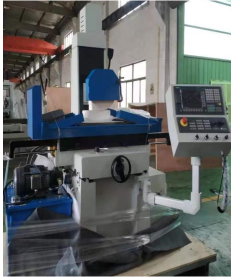
Figure 3: Hydraulic sliding X-axis, servo-driven Y-axis, and servo-driven Z-axis mechanism
