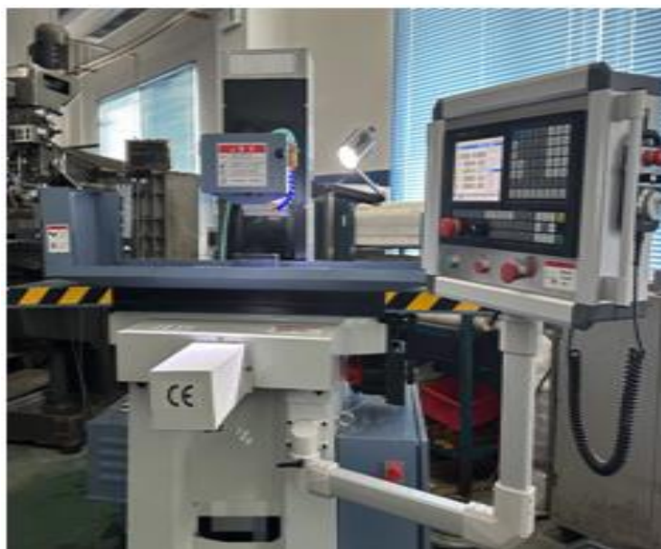
Figure2: Servo-driven X-axis, servo-driven Y-axis, and servo-driven Z-axis mechanism
